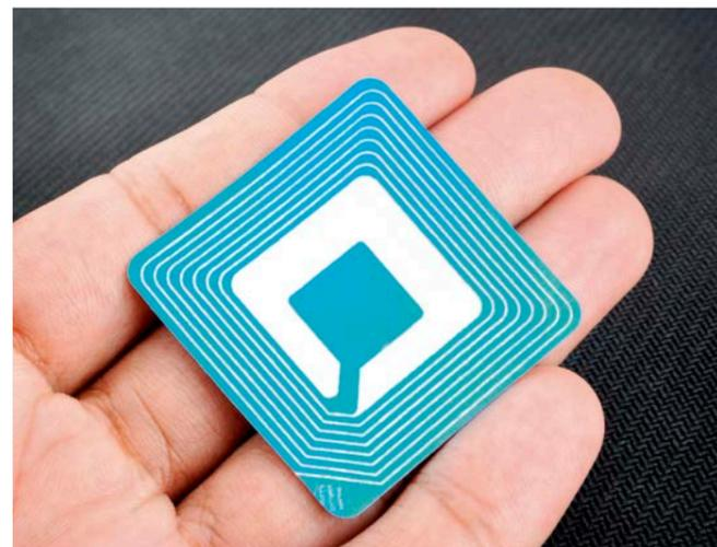
Another type of labels used in the identification of assets are **RFID** tags that allow remote and contactless identification of the assets.
