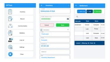
The AMS OPTIEST application for the inventory of fixed assets is based on the RFID technology. It enables tracking of fixed assets using special tags that are placed on the products. The reader captures the data using radio waves collected by the system to monitor and immediately take action if need be. Automating the processes of fixed asset monitoring in the company using RFID results in numerous benefits.
